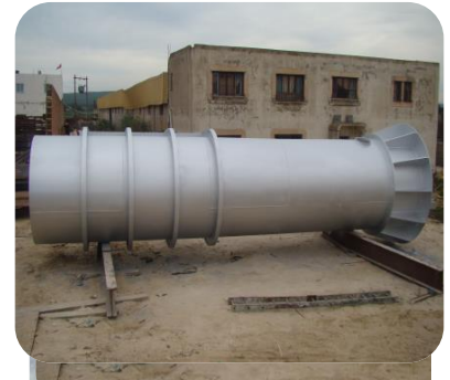
2010: Chimney length: 20m Ø: 2m CORTEN steel - CPG
