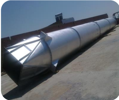
2010: Chimney length: 60m Ø :2m- SOTACIB
